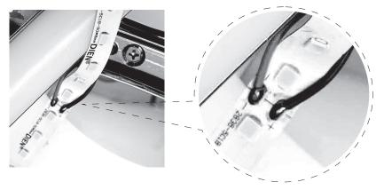
Using a soldering iron, disconnect the LED strip from the fitting.
